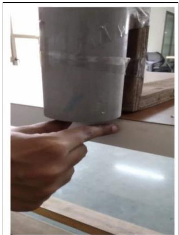
Fig 2: Finger positioning during ruler drop test method
