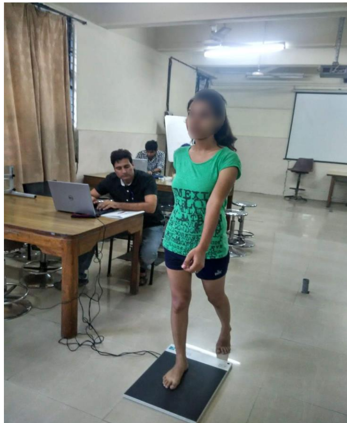
Fig 2: Picture of a Subject While Rolling Over the Pressure Plate During the Collection of Data
