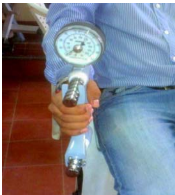
Fig 7: Standard position for recording pain free grip strength using a hand-held dynamometer
