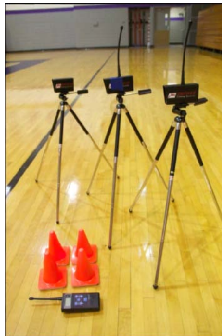
Fig 1: Equipment includes: laser transmitters and receiver, extendable tripod stands, and handheld remote storage and data recorder device.
